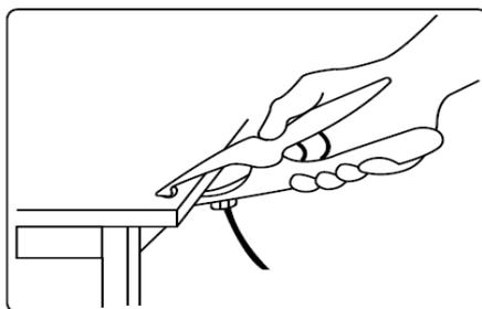
**CAUTION:** DO NOT TAP the electrode on the piece as the coating could be damaged, making it more difficult to attract the arc. Once the arc is achieved, try to maintain a distance from the piece equivalent to the diameter of the electrode used, and keep this distance as constant as possible during welding, remembering that the forward inclination of the electrode must be between 20 and 30 degrees.
