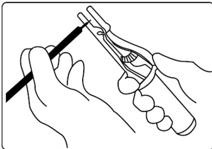
Fix the uncoated end of the electrode in the electrode holder and connect the ground clamp to the piece to be welded, always ensuring proper electrical contact. Cover your eyes and face with the protection screen and try to rub the tip of the electrode on the piece to be welded, following a movement as if you wanted to light a match; This is the most correct method to generate the arc. Replace the electrode when its tip is only 2-3 cm away from the electrode holder.
