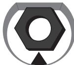
Cuchilla perpendicular a la cara de la tuerca / Perpendicular blade against the face of the nut.
