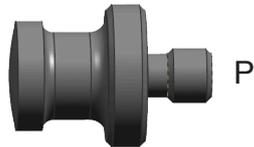
**NOTE:** Make sure that the point "P" is tightened against the piston road.
